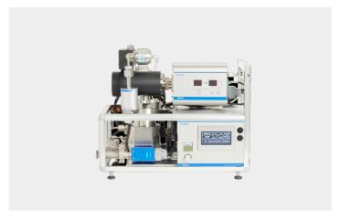
The Qulee RGM2-201 F reactive process gas monitor is a process monitor with a differential exhaust system that supports reactive gases such as etching, CVD and ALD equipment of the Qulee series. With the unique ion source and exhaust system structure of Alvac, it has excellent corrosion resistance for reactive gases and can be measured stably for a long time.
